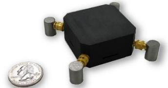
The sensor to the right comprises the DIDS Sensor Unit along with four Acoustic Emission transducers. The transducer array is designed in combination with the extremely low-latency trigger capability to insure that the entire trigger event is captured.
