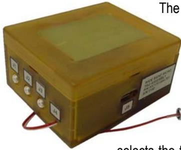
The Wide-Band Microminiature Tri-Axial Accelerometer Unit (WB MicroTAU) system is a wireless, high-speed data acquisition network for dynamic acceleration sensing and recording applications. The system includes WB MicroTAU Remote Units, a WB MicroTAU Receiver Unit, and the Graphical User Interface (GUI).
